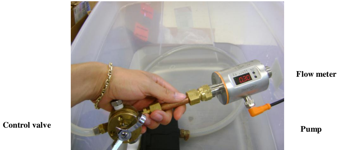
Figure 3.20: Photograph of the flow meter calibration setup developed and used in the present study.
