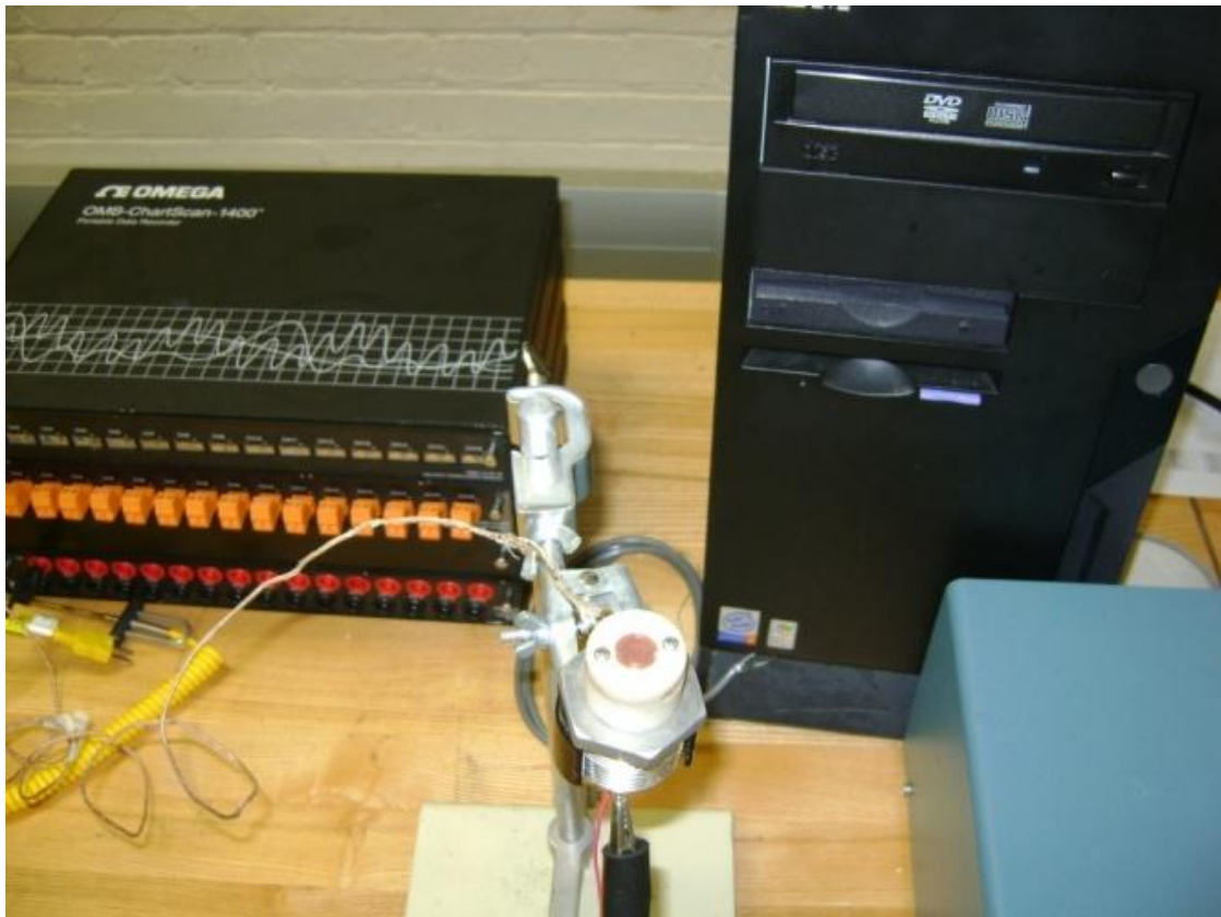
Figure 3.15: Photograph of heater testing setup.
