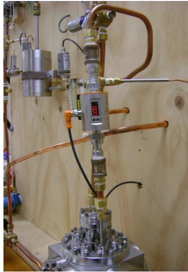
Figure 4.1: Photograph of the flow meter mounted on the liquid pipeline of the heat transfer spray cooling loop developed and used in the present study.
