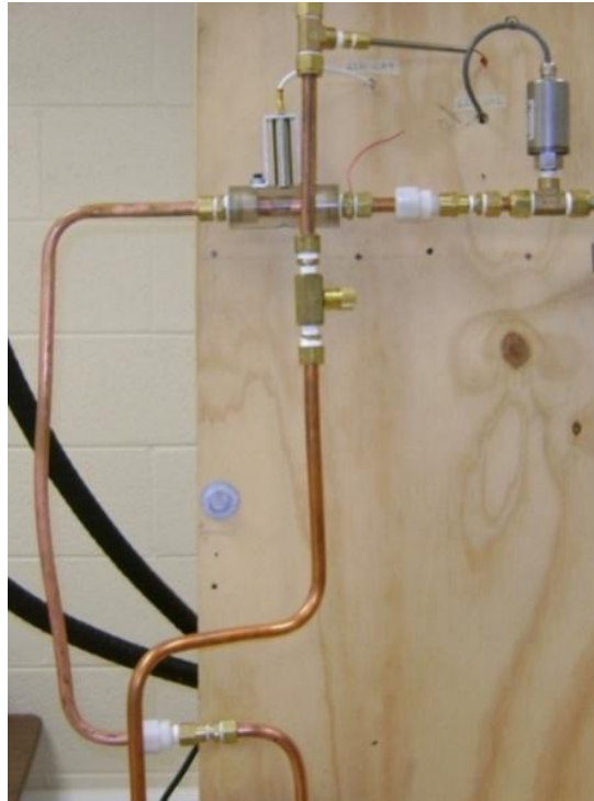
Figure 4.5: Photograph of the void fraction sensor installed in the heat transfer loop developed and used in the present study.
