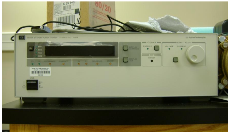
Figure 3.3: Photograph of the Agilent Technologies 6030A power supply.
