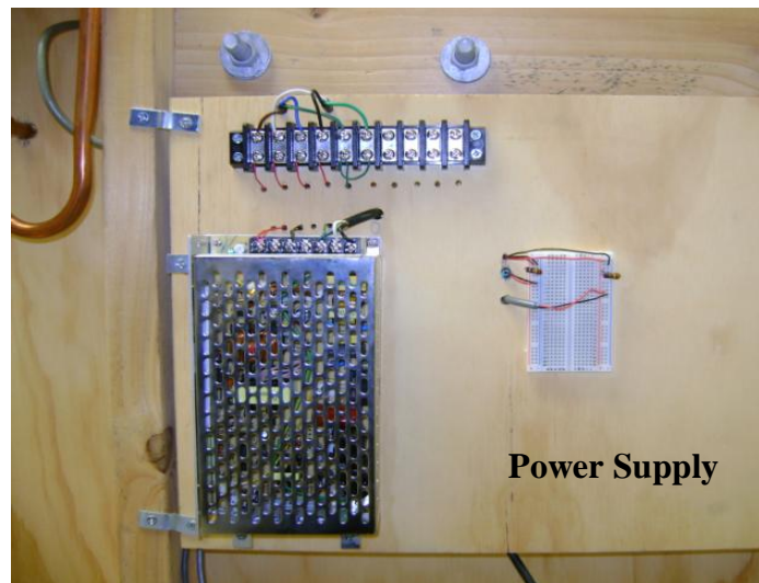
Figure 3.4: Integrated Power Designs SRW series power supply.
